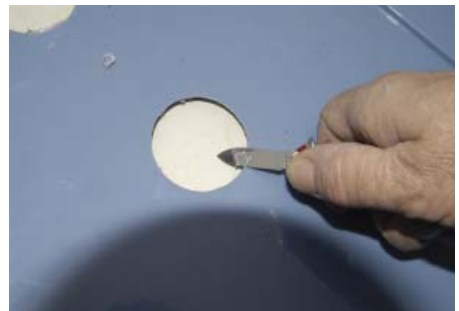
6. Make the holes in the reservoir lid big enough for the bottom of the fill/drain and overflow fittings to fit through.
