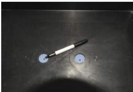
5. Once holes are drilled, set nursery flat over the top of the reservoir. Mark a bull's-eye in the middle of each hole. These marks will serve as the center of the holes in the reservoir lid.
