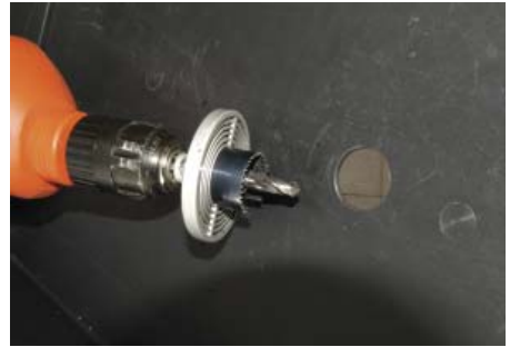
4. Use a hole drill bit to cut a hole in the bottom of the nursery flat.
